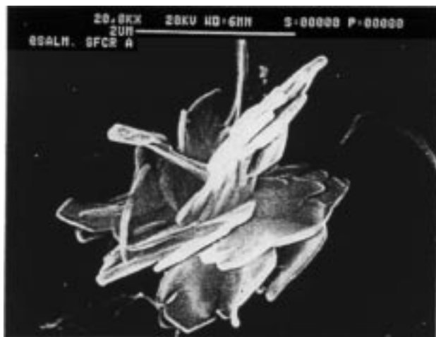
Figure 10. Scanning electron micrograph of SEDS prepared salmeterol xinafoate from acetone solution at 50 °C and 200 bar.
